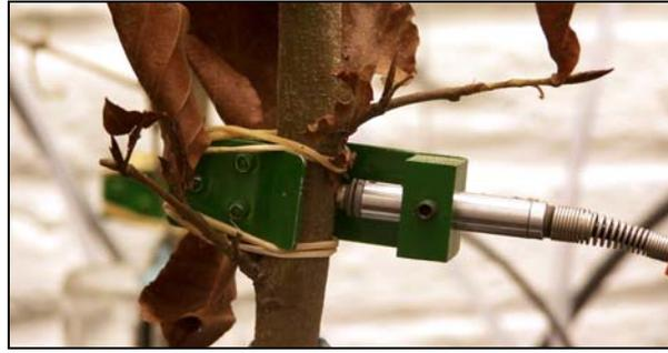
**Figure 2.15:** A linear variable displacement transducer (LVDT) installed on a young beech stem and supported by a custom-made stainless steel holder.
