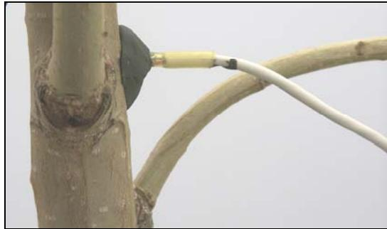
**Figure 2.17: A thermocouple psychrometer sensor inserted in an eastern cottonwood stem. The sensor is sealed to the stem surface with flexible putty adhesive.**
